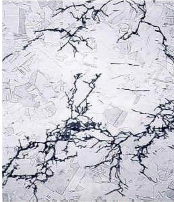
SCC in a 316 stainless steel chemical processing piping system; photo courtesy https://www.nace.org/Corrosion-Central/Corrosion-101/Stress-Corrosion-Cracking-(SCC)/
