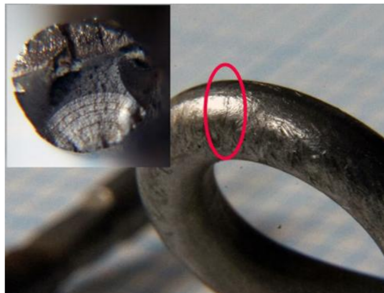
SCC in a 316 stainless steel chemical processing piping system; photo courtesy https://www.nace.org/Corrosion-Central/Corrosion-101/Stress-Corrosion-Cracking-(SCC)/
